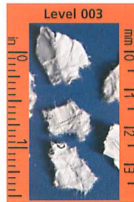
This Security Level is suggested for most common commercial shredding jobs. Similar to Level 3 Security Level DIN 32757. Combines an excellent degree of security, bulk reduction of shredded material and shredding output. Shredding output 300-320 Kg. (670-715 lbs) per hour.
