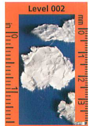
Low degree of bulk reduction of shredded paper. Shredding output 400-420 Kg. (900-940 lbs) per hour.
