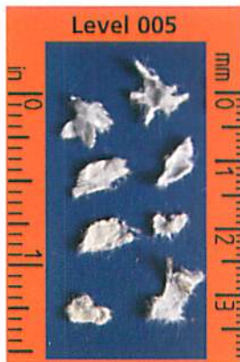
High Security, suitable for Embassies, Military and Government offices. Similar to Level 5 Security Level DIN 32757. Very high bulk reduction of shredded material. Shredding output 100-120 Kg. (225-265 lbs) per hour.
